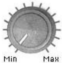
The **MOD CTRL** knob allows you to control the amount of **frequency modulation** that is applied to the generator. The modulation source has to be entered in the « MOD» input. This can be any kind of signal (e.g. output of second generator).
