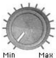
You can control the cut-off frequency using the **FREQUENCY** knob. Far left position closes the filter for incoming frequencies, far right opens the filter entirely for all incoming frequencies.
