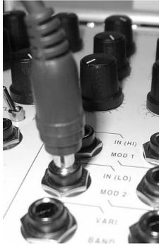
The input of the WaveX is hard patched to the 2<sup>nd</sup> filter input (see the picture to the left).
